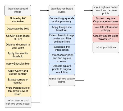
Figure 7: Overview of image processing pipeline
