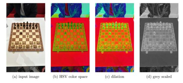
Figure 9: HSV dilation process
