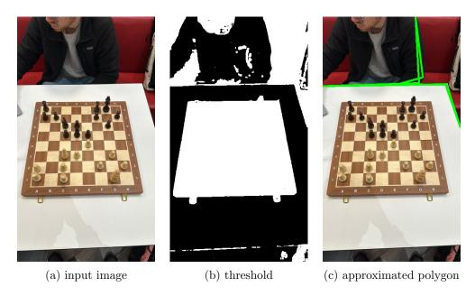
Figure 18: Failure to detect chessboard in image of second dataset due to chessboard not being the largest contour in the image
