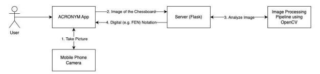
Figure 2: System Architecture and Interaction Diagram
