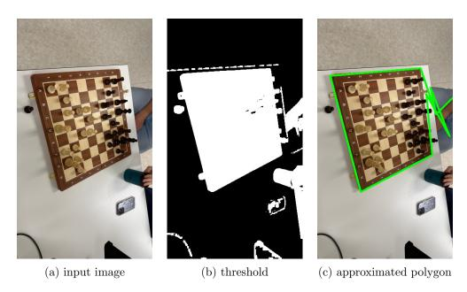
Figure 16: Failure to detect chessboard in image of first dataset due to table corner too close to the chessboard
