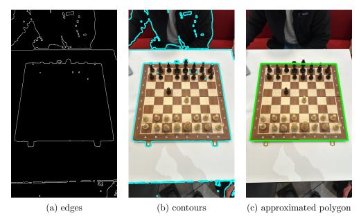
Figure 11: Steps from edge detection to board corners
