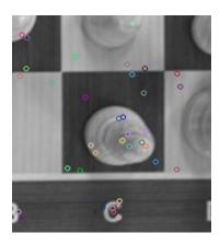
Figure 20: Identified key points using SIFT
